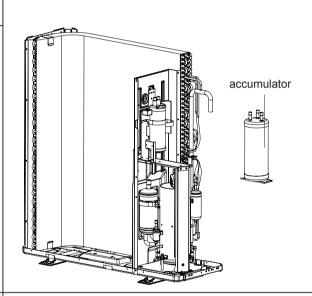
19. Remove gas-liquid separator
