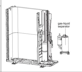
20. Remove supporting board and supporting board sub-assy
