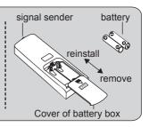
3. Reinstall the cover of battery box.
