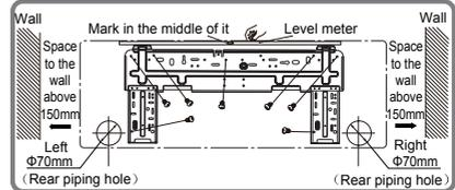
2. Open a piping hole with the diameter of Φ55 or Φ70 on the selected outlet pipe position. In order to drain smoothly, slant the piping hole on the wall slightly downward to the outdoor side with the gradient of 5-10°.
