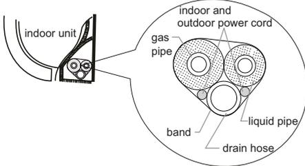
2. Reserve a certain length of drain hose and power cord for installation when binding to a certain degree, separate the indoor power and then separate the drain hose.
