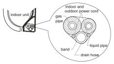
Reserve a certain length of drain hose and power cord for installation when binding them. When binding to a certain degree, separate the indoor power and then separate the drain hose.
