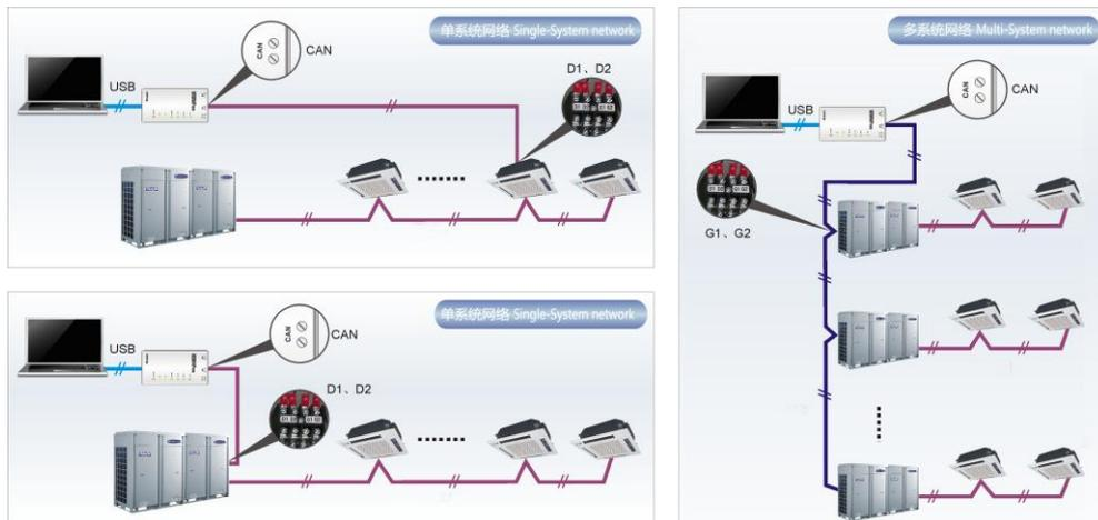
It can be connected with single-system network or multi-system network. In the single-system network, indoor units or outdoor units are connectable, while in the multi-system network, only the master outdoor unit can be connected.
