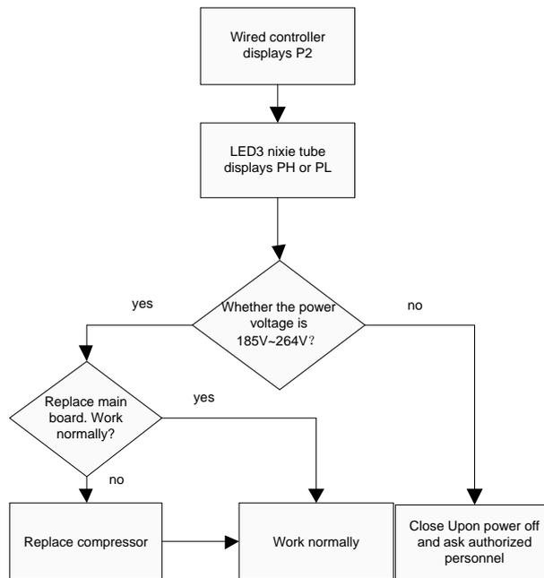
(17) AC current protection for inverter compressor
