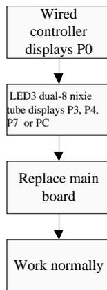
(10) Drive IPM overtemperature protection for compressor
