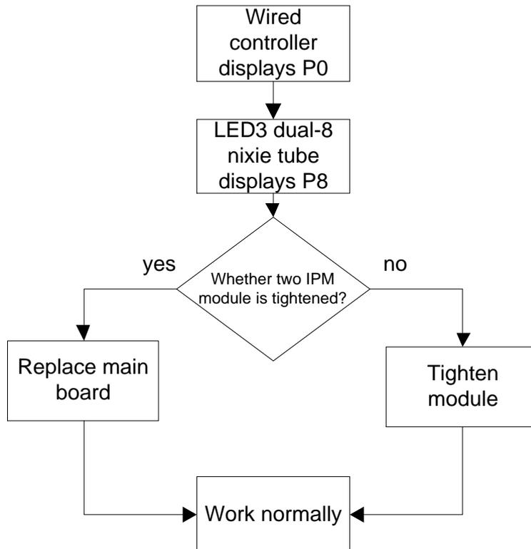
(11) Desynchronizing protection for inverter compressor
