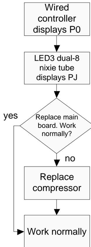
(13) Loop malfunction of driven charging for compressor
