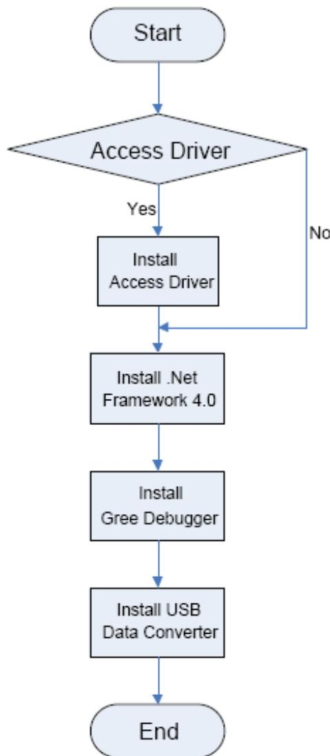
This flowchart describes basically the software installation process. See below for details.
