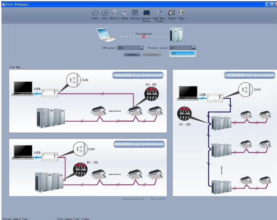
After the selection, click “Connect”. If units can communicate normally with computer, then the interface of numbers will be shown soon. Otherwise, “Connecting” will be shown.
