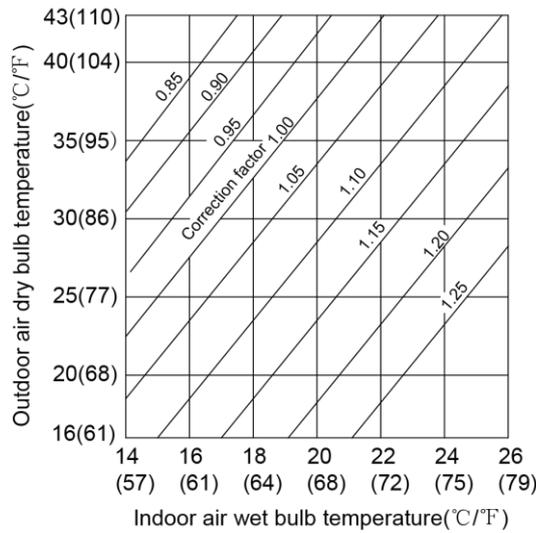
(2) Correction factor of heating capacity
