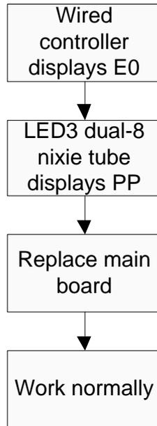
(18) Communication malfunction between main controller and driver of inverter compressor
