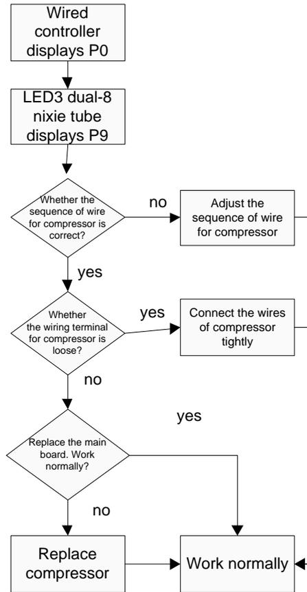
(12) Failure startup for inverter compressor
