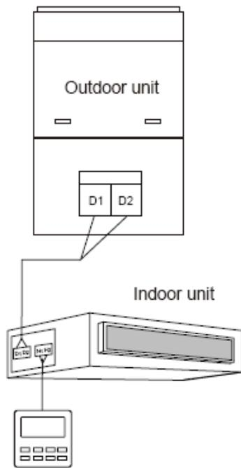
Fig. 2.2.4.1 One wired controller control one indoor unit
