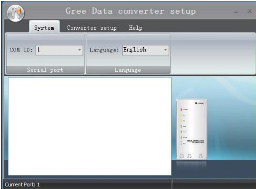
Select the function that is to be set and the corresponding baud rate (refer to the look-up table) in the “Converter Setup”. Then click “Set”.
