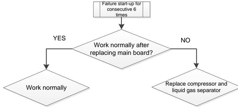
(9) Reset protection for drive module of compressor, drive PFC protection for compressor, malfunction of drive temperature sensor for compressor, circuit malfunction of drive current detection for compressor
