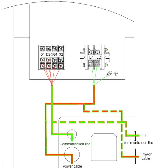
There are two wiring diagrams for communication wires of indoor/outdoor units and remote monitor:
