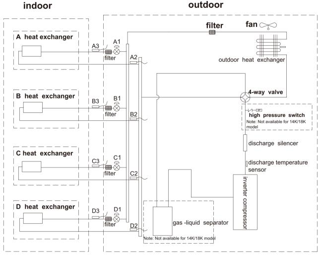
A1:A-unit electronic expansion valve B1:B-unit electronic expansion valve
