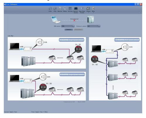
COM selection: the serial port in your computer can be detected automatically. You just need to select your desired serial port.
