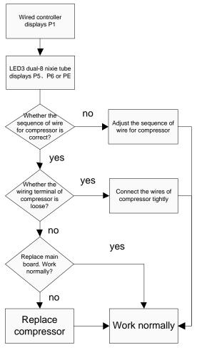
(16) High pressure protection for driven DC bus bar of compressor, low pressure protection for driven DC bus bar of compressor
