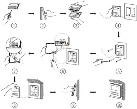
Fig. 3.7 Installation diagram for wired controller
