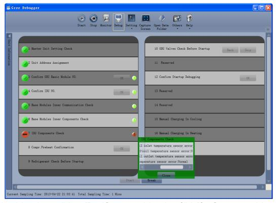
During debugging, a click on "Break" can stop debugging. Click "Start" to resume debugging and
