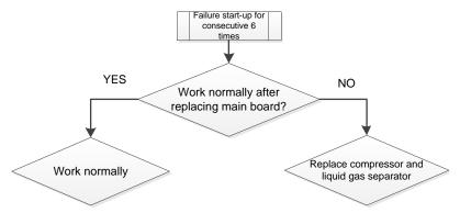
(9) Reset protection for drive module of compressor, drive PFC protection for compressor, malfunction of drive temperature sensor for compressor, circuit malfunction of drive current detection for compressor
