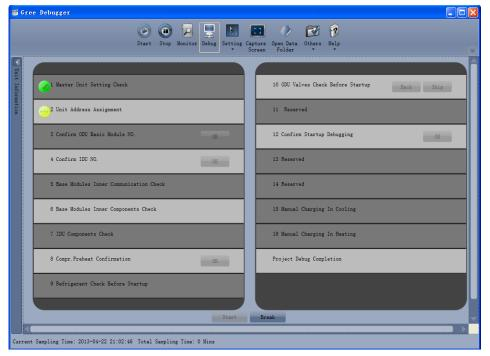
If "OK" button is displayed, it means user needs to judge whether to continue debugging or not. Click icon and relevant information will be shown for your reference. Click "Close" to close the pop-up (For No.3 Confirm ODU Basic Module NO. and No.4 Confirm IDU NO., the current number of units under debugging will be displayed. See the following marked with circle. For No.8 Compr. Preheat
