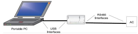
HBS, CAN and RS485 of the converter can be switched by buttons. Press the button "SET" on the converter to realize the conversion among HBS, CAN and RS485 interfaces. You can check the setting through the function LEDs.
