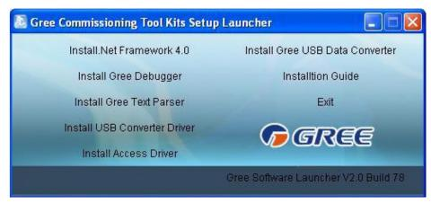
For the first time to use Gree Commissioning Tool Kits, install these programmes: .Net Framework 4.0, USB Data Converter, Access Driver (necessary for versions below OFFICE 2007), Gree Debugger.
