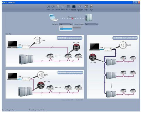
Protocal selection: This is to select the communication method of your units. Currently, CAN is applicable to the units.
