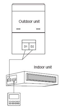
Fig. 2.2.4.1 One wired controller control one indoor unit
