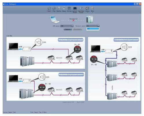
After the selection, click "Connnect". If units can communicate normally with computer, then the interface of numbers will be shown soon. Otherwise, "Connecting" will be shown.
