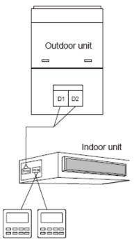
Fig. 2.2.4.2 Two wired controllers controls one indoor unit
