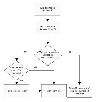
(17) AC current protection for inverter compressor
