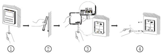
Fig.2.1.3 Removal of Wired Controller
