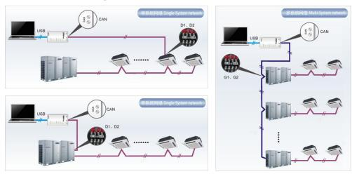
It can be connected with single-system network or multi-system network. In the single-system network, indoor units or outdoor units are connectable, while in the multi-system network, only the master outdoor unit can be connected.
