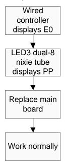
(18) Communication malfunction between main contoller and driver of inverter compressor
