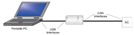
Gree monitoring software should be connected with RS485 interface when converter is used. Connect outdoor or indoor units or the mainboard of wired controller according to actual needs.
