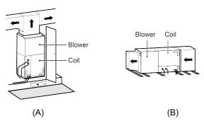
Based upon the actual conditions, Multi-Position A-Coils come factory installed with a vertical and horizontal drain pans and can be configured for upflow or horizontal pull-through installations.
