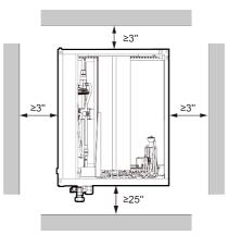
When installing in an area directly over a finished ceiling (such as an attic), an emergency drain pan is required directly under the unit. See local and state codes for requirements. When installing this unit in an area that may become wet, elevate the unit with a sturdy, non-porous material. In installations that may lead to physical damage (i.e. a garage) it is advised to install a protective barrier to prevent such damage.
