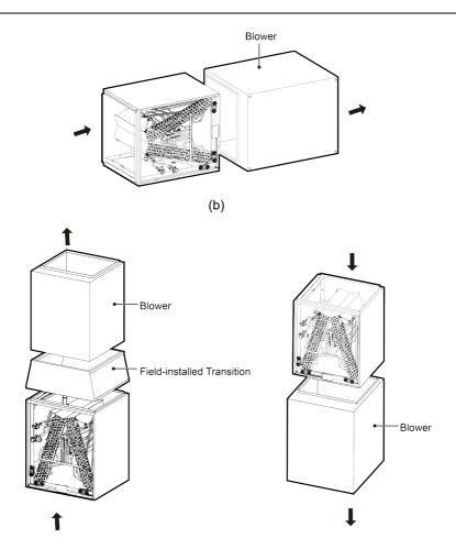
If the air inlet of blower is different with the air outlet of coil in size, it may be necessary to install a field-installed transition between the blower and the coil to proper airflow distribution (as shown in figure (a)).
